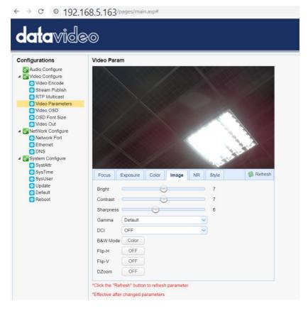
The Image option allows users to set several parameters including Bright, Contrast, Sharpness, Gamma, DCI, B & W Mode, Flip-H, Flip-V and DZoom.
